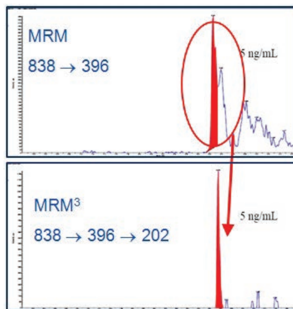
Figure 4. MRM 3 Significantly Improved Selectivity of Detection in Plasma. Elimination of chromatographic interferences and background noise improves the LOQ for exenatide in plasma.
