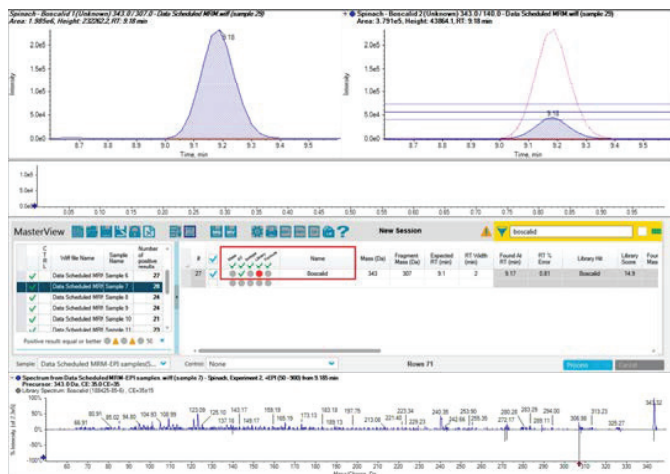
Figure 11. Boscalid was detected in a spinach samples with a concentration of 14.9 µg/kg, the ion ratio of 21.3 is inside the 30% tolerance (top), however, the MS/MS library searching with a PUR of 14.9% indicated strong matrix interference and suggest that Boscalid is not present in the sample (bottom)
